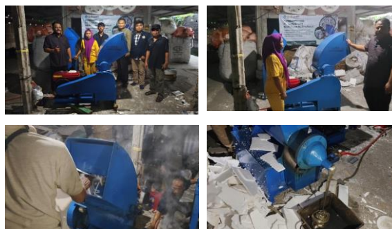
Figure 3. Training and Mentoring on the Operation of the Appropriate Technology Styrofoam Melting Machine.
